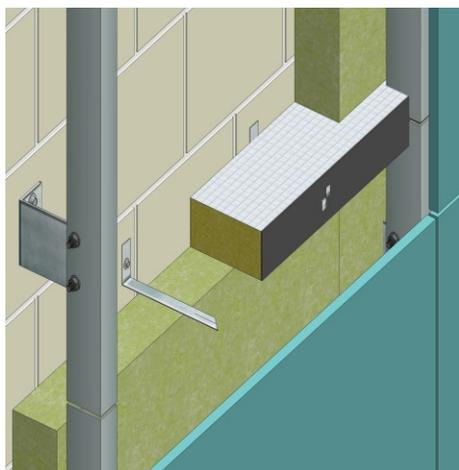
Rainscreen cladding systems typically incorporate a minimum 25mm<sup>(1)</sup> continuous ventilated air space. The inclusion of this cavity ensures that any rain penetration can drain freely within the façade construction.
